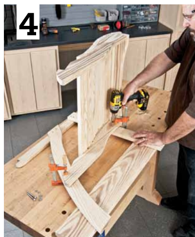
▲ Attach the seat assembly to the two leg assemblies with 1-5/8-in. screws.
