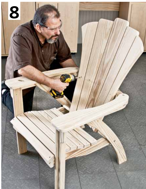
▲ When assembling the back, work from the center out and from the top down.
