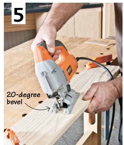
▲ Angle the jigsaw base and cut the beveled curves in one pass. Move slowly around the faceted corners.
